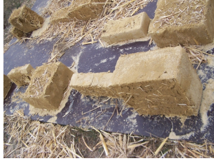
(a) Brick with fibres ( 1\ 200\ \text{kg.m}^{-3} )
